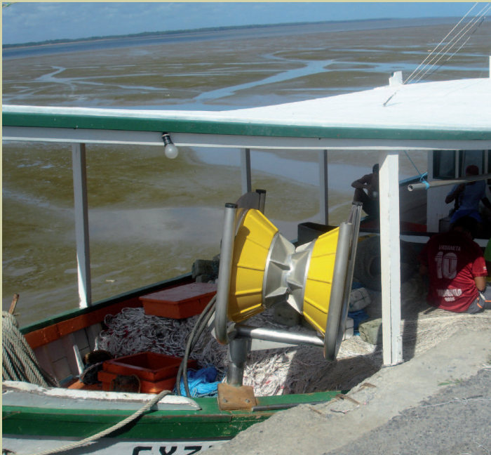
EQUIPMENT: A netter in Guyana with a Virhydro net hauler on the gunwale. "We don't sell many spare parts. The knives are reversible so they can be used twice, but still have to be replaced eventually," Isabelle Blancard said. "But in general, there isn't a great deal to do in after-sales."
