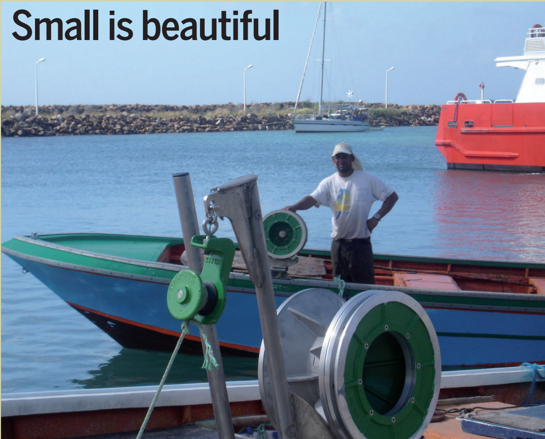
DEVELOPMENT: A traditional Saintoise fishing boat in the French West Indies fitted with a Virhydro combined net and pot hauler, powered by a small hydraulic powerpack
